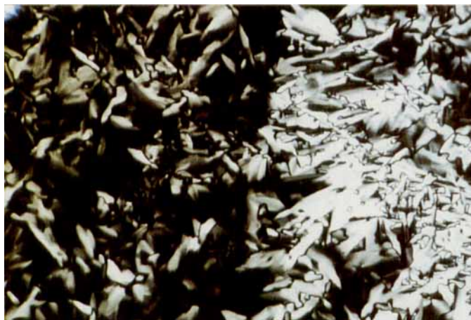
Figure 5. Contact preparation of D-ribose-di- n -decyl-S,S-acetal (right) and 18 (left) suggesting complete miscibility (crossed polarizers, 55°C).
